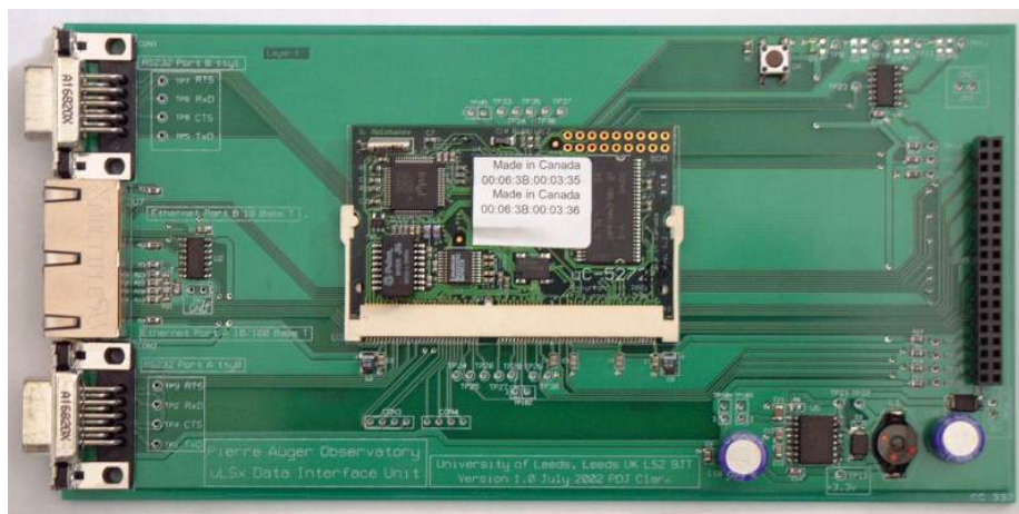
Figure 3.1.7 : Micro-LSX unit provides E1 to TCP/IP conversion
