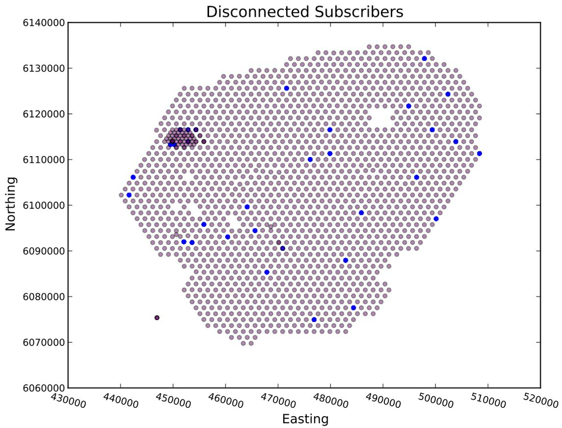
Figure 11: This map shows in blue what subscribers are listed as disconnected in the "Disconnected Subscribers Report" section of the SYSTEM~1.TXT files on a normal operation day. The mauve shows the location of subscribers not listed in the report and is used to aid interpretation of the map.
