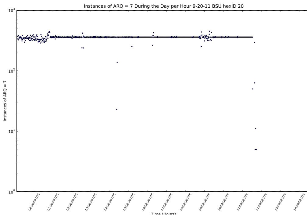
Figure 4: The count of ARQs reaching level 7 per minute for BSU 32 on September 20, 2011. Maximum number of ARQs that can be reported per minute by the array is 360 reports.
