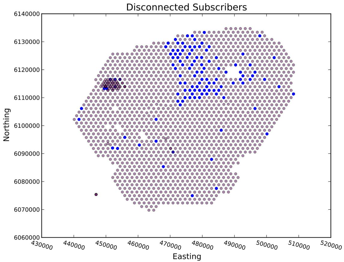
Figure 12: This map shows in blue what subscribers are listed as disconnected in the "Disconnected Subscribers Report" section of the SYSTEM~1.TXT files on the ARQ spike day of September 20, 2011. The mauve shows the location of subscribers not listed in the report and is used to aid interpretation of the map.
