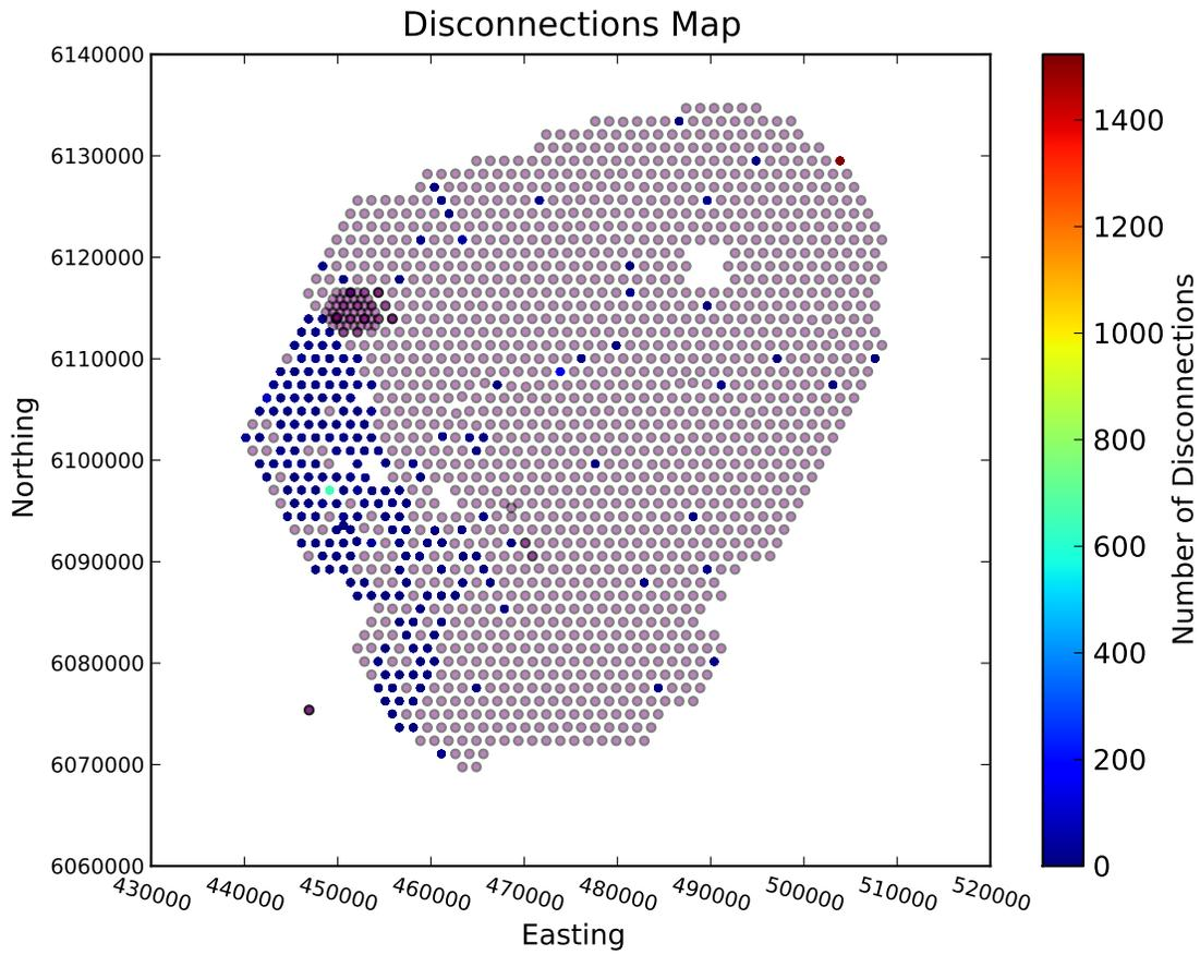
Figure 13: This map shows which subscribers are listed and the number of disconnections reported in the "Link Disconnections Report" section of the SYSTEM~1.TXT files. The mauve shows the location of subscribers not listed and is used to aid interpretation of the map.
