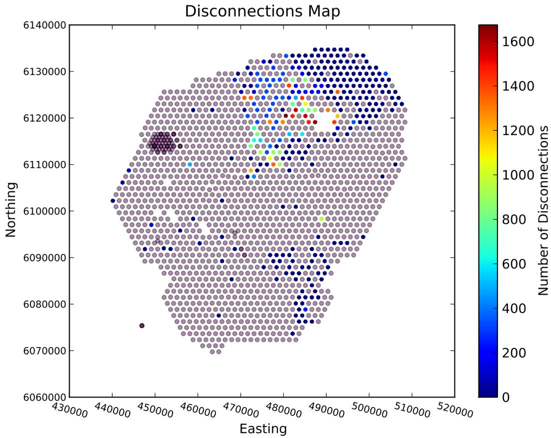
Figure 14: This map shows which subscribers are listed and the number of disconnections reported in the "Link Disconnections Report" section of the SYSTEM~1.TXT files. The mauve shows the location of subscribers not listed and is used to aid interpretation of the map.
