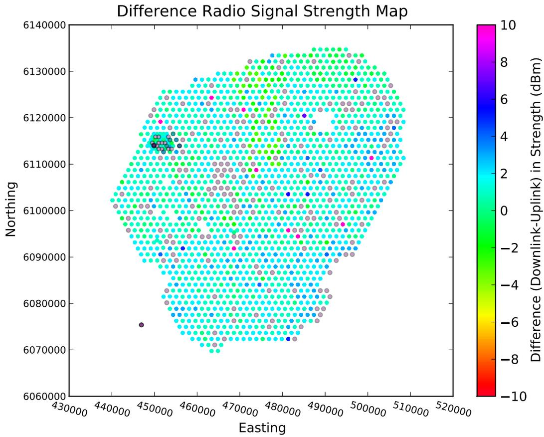
Figure 17: This map shows the difference between the reported downlink and uplink (downlink minus uplink) signal strength of the subscribers on a typical day. Points represented in mauve show the location of subscribers reporting no signal strength data.
