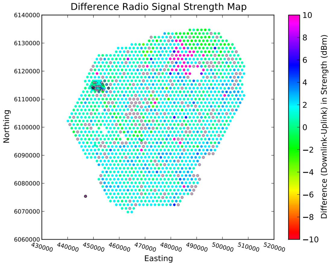
Figure 18: This map shows the difference between the reported downlink and uplink (downlink minus uplink) signal strength of the subscribers on an ARQ spike day. Points represented in mauve show the location of subscribers reporting no signal strength data.
