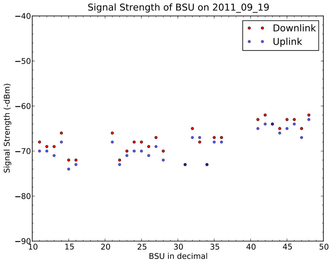
Figure 7: The signal strength as reported by the BSUs. The red markers represent downlink signal strength. Blue markers represent uplink signal strength. Large gaps between the two indicate problems in one of the signals.
