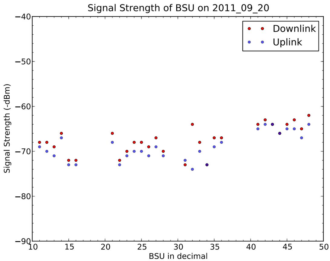
Figure 8: The signal strength as reported by the BSUs. The red markers represent downlink signal strength. Blue markers represent uplink signal strength. Large gaps between the two indicate problems in one of the signals.
