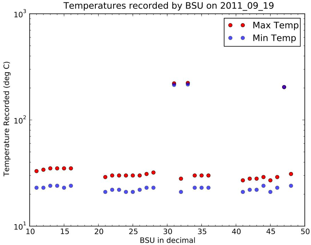
Figure 9: The report of the minimum and maximum temperatures at the BSUs in Celsius on September 19, 2011. The red markers represent maximum temperature. Blue markers represent the minimum temperature.
